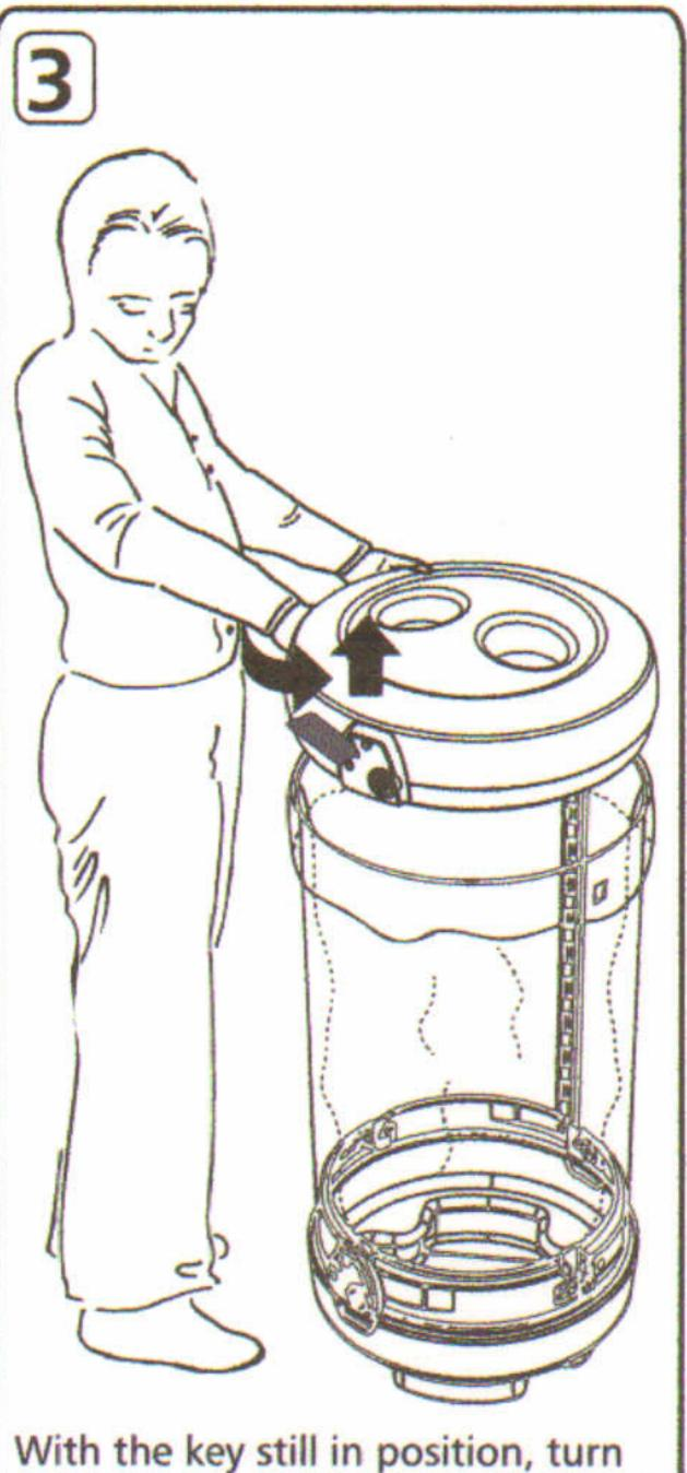
hood anti-clockwise, then lift hood off. Remove the key .
