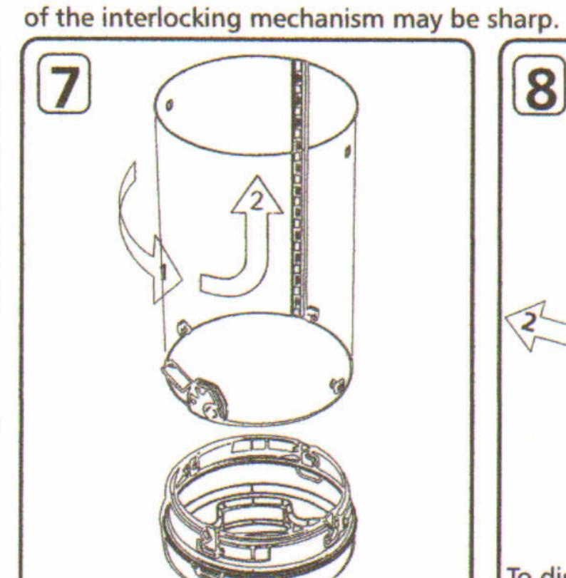
Hold the body with both hands, twist anti-clockwise and lift away from the plinth. Remove the key and keep safely.
