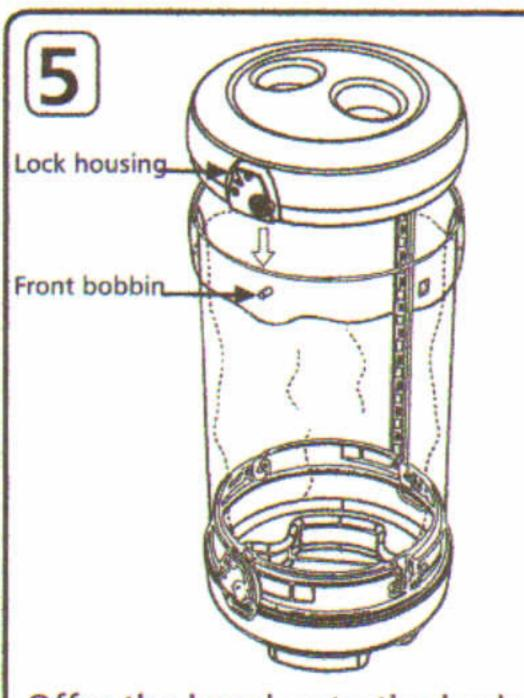
Offer the hood onto the body and align the lock housing with the front bobbin by turning the hood. Push the hood firmly downwards to automatically lock the bin.
