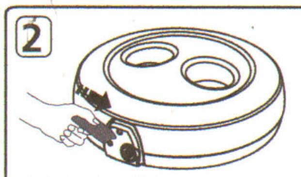
Push the key all the way into the lock. (Do not turn the key.) This will automatically release the locking mechanism.
