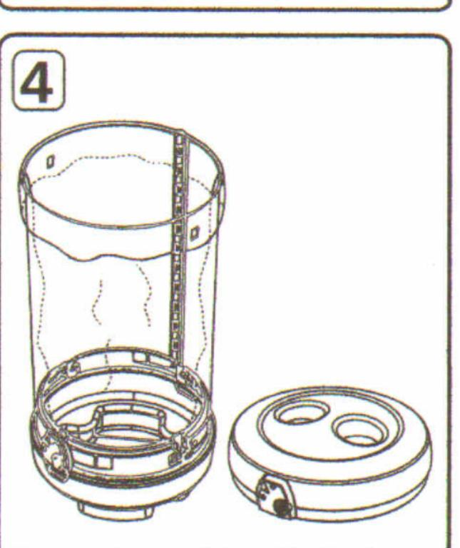
Place a clear sack into the body and hook over the rim with approximately 100mm overhang.
