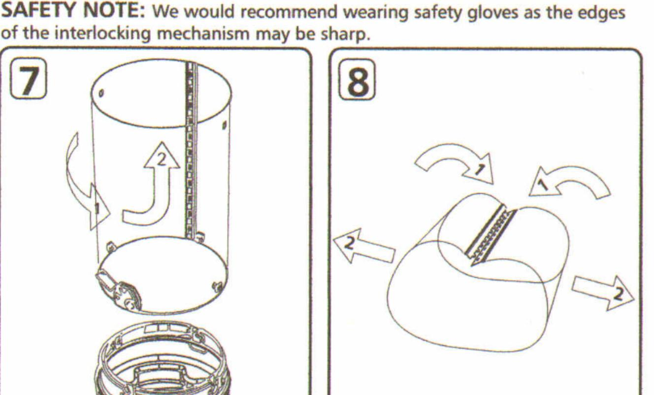
To disassemble the body place on a well protected and soft surface, joint uppermost. Push down either side of the interlock to disconnect the tabs, and allow the sheet to spring flat.
