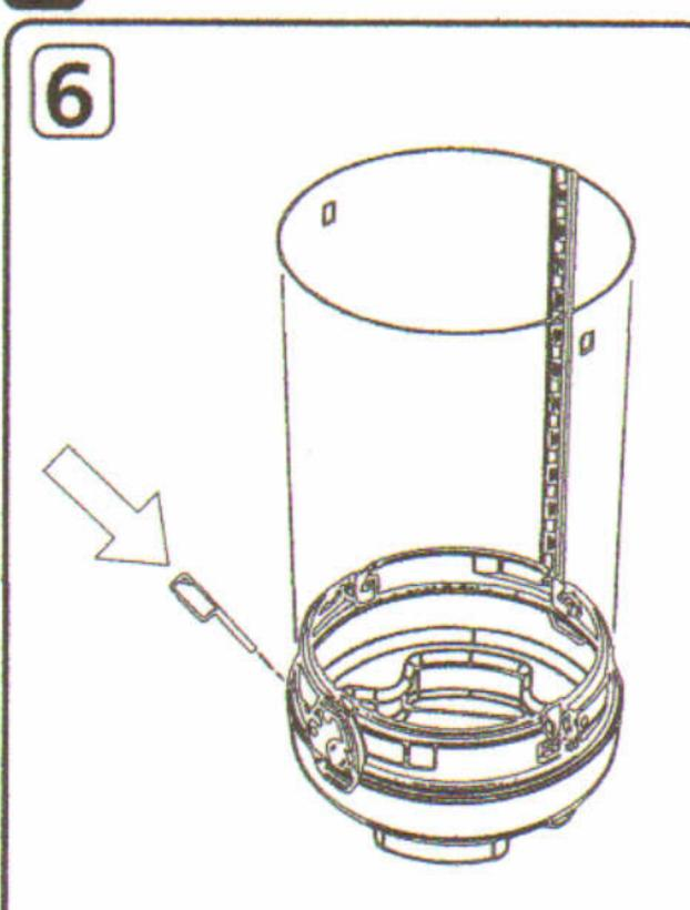
Remove hood as (1) above, remove sack if present. Insert the plastic key into the lock.
